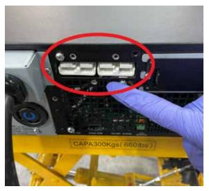
J. Connect external battery pack to UPS using the plugs on the chassis. Please note the connector with blue and white wires goes into the socket near the power cord, and the connector with black and red wires goes into the socket near the network card. Please refer to the following 2 pictures.
