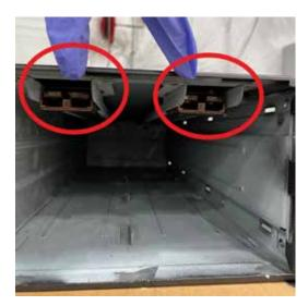
PLEASE NOTE: The following picture demonstrates a wrong way of handling the battery pack. Do NOT move or install battery packs by grabbing the connector or wires.
