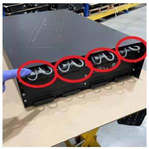
H. Locate the external battery pack connector on the back of UPS by removing the cover.
